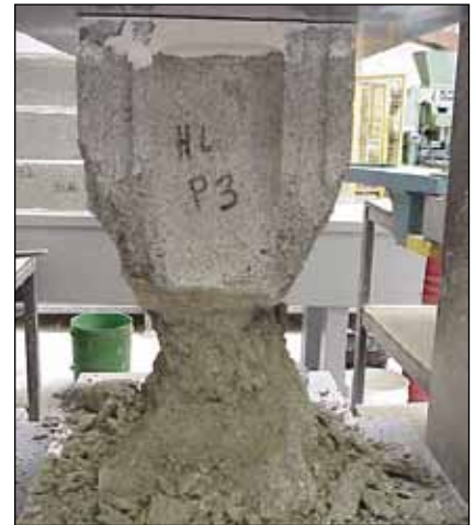
Prism specimen following compression testing.
