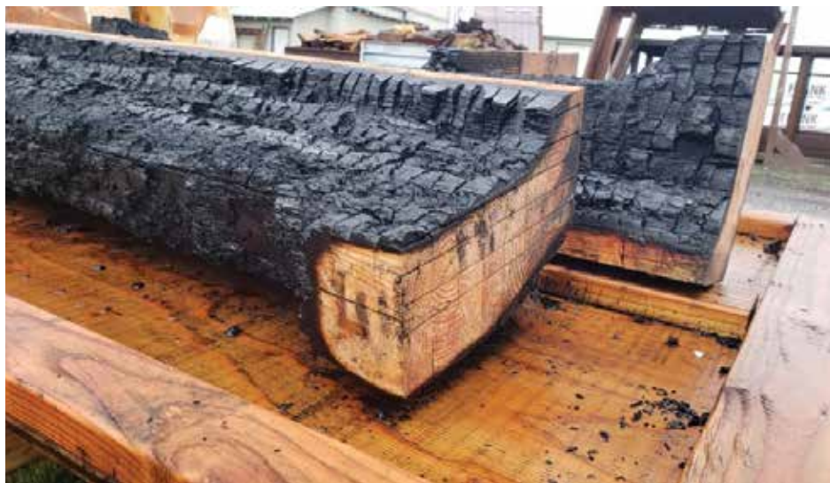
Figure 5. Uncharred bearing interface on the bottom of the beam after a 2-hour fire test.
