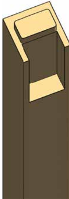
Figure 1. End column with beam bearing pocket.
