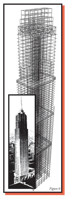
target periods for the building, satisfying the motion comfort criteria. As a result of these studies, preliminary planning now allows for a Tuned Mass Damper to be included in the early planning and cost allowances. This tower is being designed in association with KLA of Colorado
