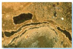
Figure 3: Transmitting Light Photomicrograph of crack in line-sand mortar healed with later calcium carbonate or calcite. (Width of photomicrograph 3.94 mm. Photography courtesy of Dr. B. Middendorf, Kassel University, Germany)
