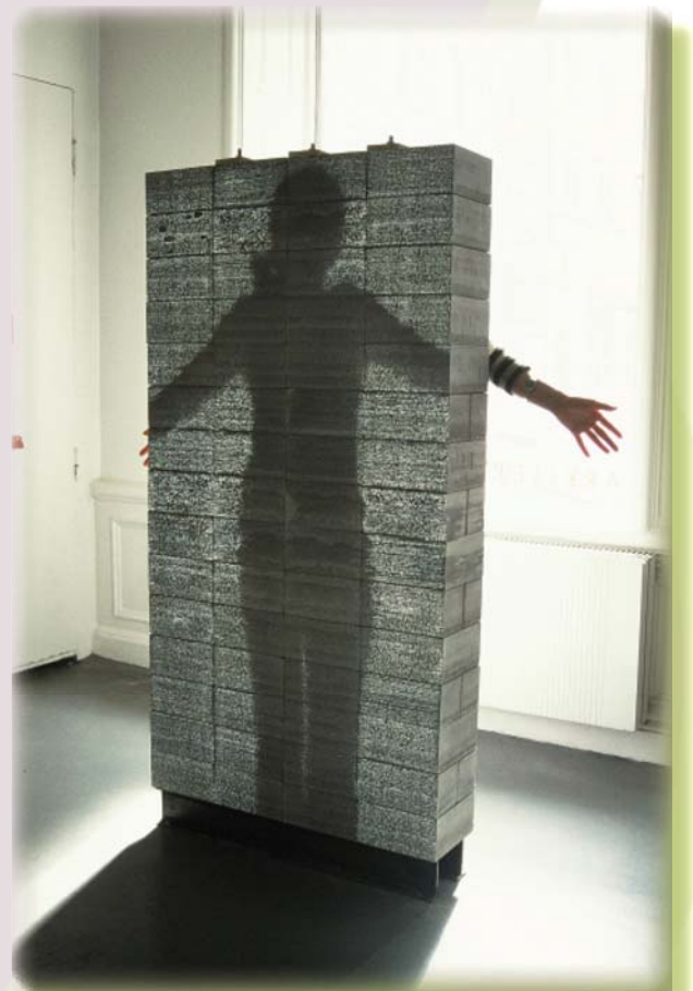
Prototype wall of LiTraCon, a translucent concrete product. Courtesy of LiTra Con, © GmbH
