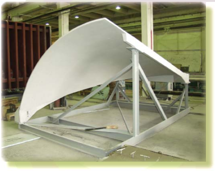
A prototype of a canopy for the Shawnessy Light Rail Transit station in Calgary, Canada, made of an ultra-high-performance concrete called Ductal. Photo courtesy of Lafarge
