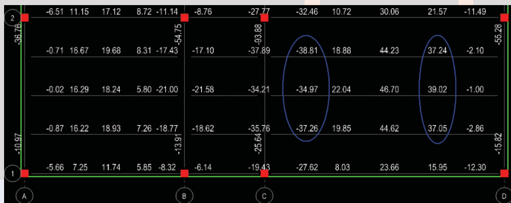
Figure 4 - As can be seen 3 parallel beam lines will have nearly at 10% different in design moments due to their location on the supporting girders
