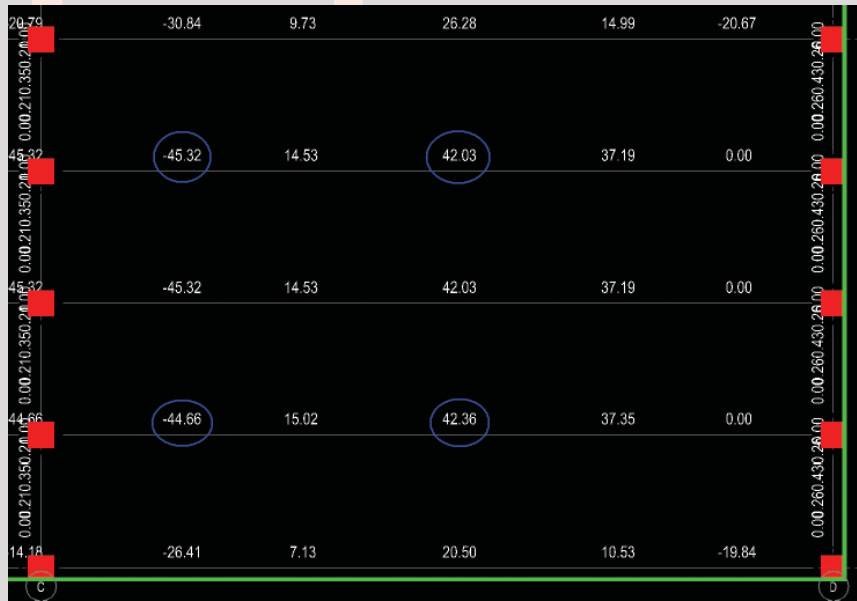
Figure 9 - These are the same spans as Figure 8 and modeled as 2D beam lines. As you can see the difference in stiffness between beam line 3 and 5 has very little impact on the final moments.
