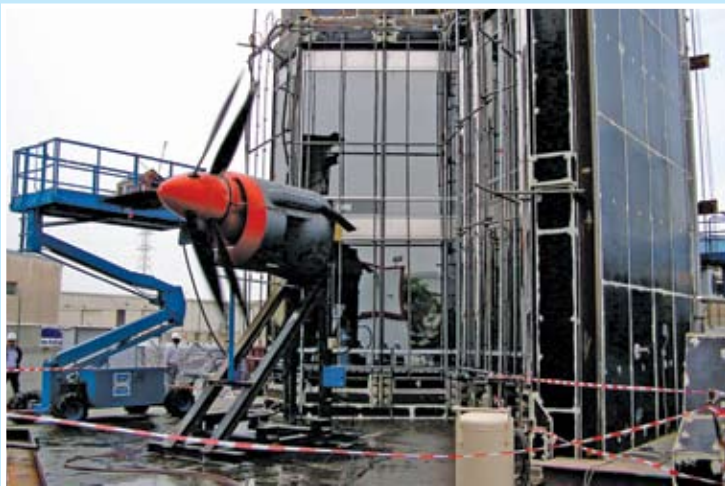
Figure 6b: Tower Test Mock-up Dynamic Test for Water Penetration
