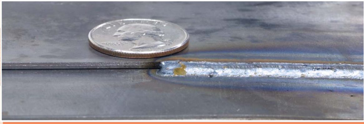
Figure 2: Gas metal arc welding can be used to make high quality welds on sheet steel.
