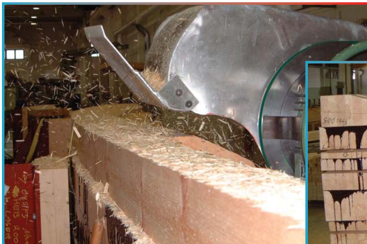
Massive computer programmed and guided grinding-cutting machine shaping the main glulam arch to the specified structural shape, size and form.
