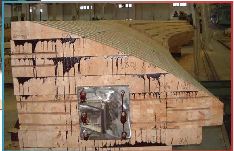
Massive computer programmed and guided grinding-cutting machine shaping the main glulam arch to the specified structural shape, size and form.
