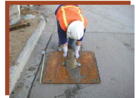
Removing slump cone and measuring slump spread.
