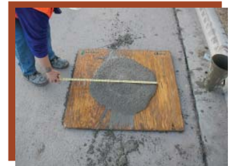
Removing slump cone and measuring slump spread.
