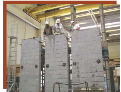
Tall masonry wall panels were built at the NCMA Labs in Herndon, Virginia, to study various aspects of self-consolidating grout, including construction and placement issues and hardened grout characteristics.
