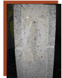
One purpose of the tall panels is to demonstrate how SCG fills less-than-ideal core spaces, such as cores containing mortar fins. SCGs are able to surround and encase mortar fins. Solidly grouted spaces are needed to develop composite action between masonry unit and reinforcement. Photo courtesy of Atkinson – Noland & Associates, Inc.
