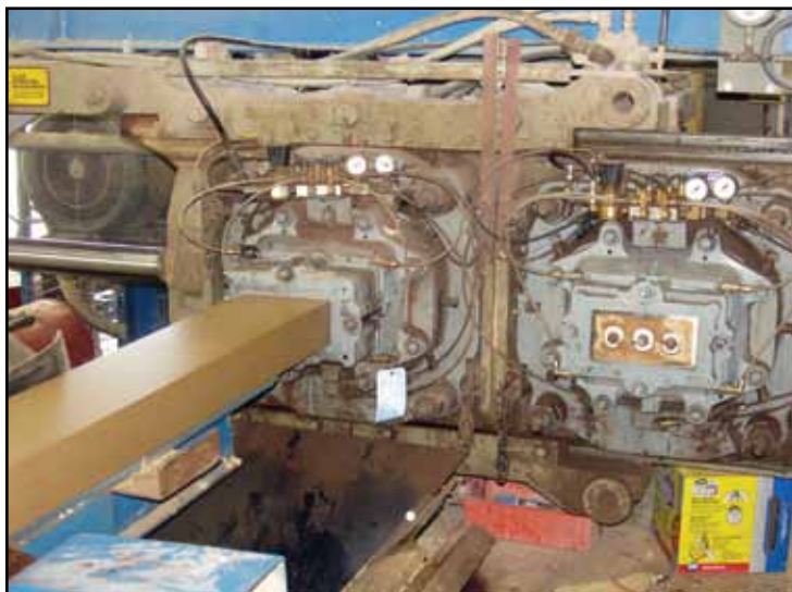
Figure 1: End of extrusion machine, with clay column before texturing and cutting for brick height, left. Adjacent die with rods that form cores in bed surface visible, right.
