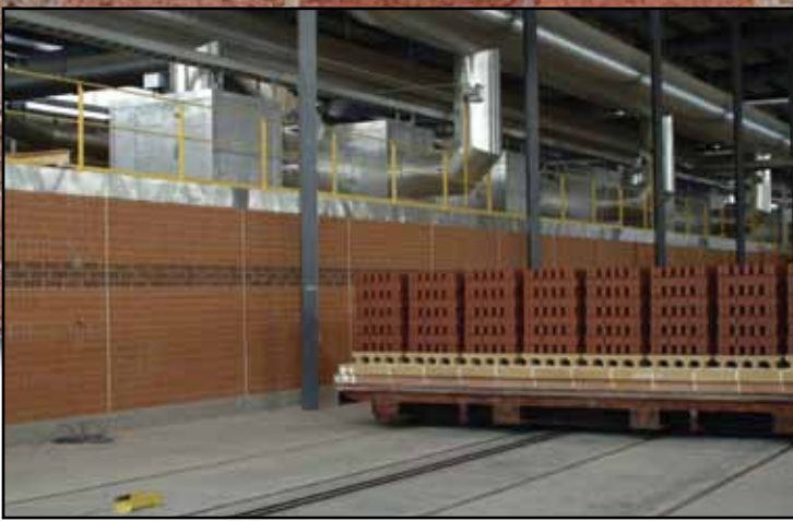
Figure 3: Extruded brick on kiln cars; tunnel kiln in background.
