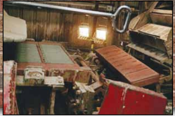
Figure 2: Molded brick in wooden molds, being rotated to remove the molds.
