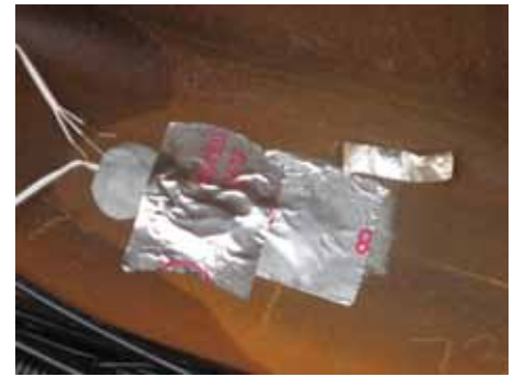
A strain gauge is installed on a prepared surface.
