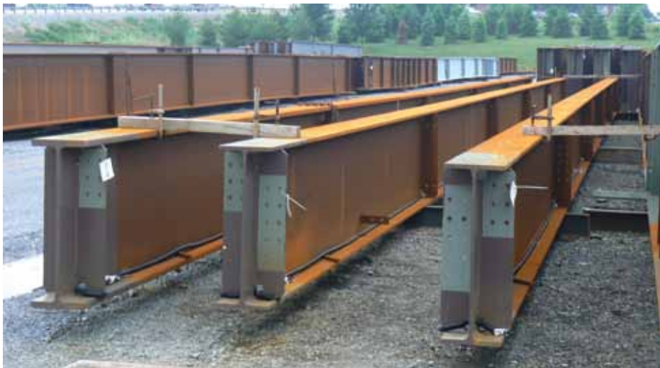
Three of the steel girders at the steel fabrication plant in Lancaster, Penn.
