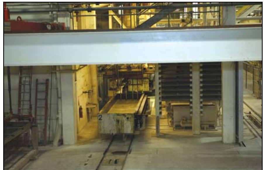
AAC rising in the mold at the AERCON production facility in Haines City, Florida. Courtesy of AERCON Florida LLC.
